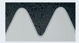
Electroless deposition (without external current) of nickel-phosphorous coatings is always uniform, even on materials possessing complex geometries. Boreholes, dents, cavities and edges are coated with very small margins of tolerance with respect to the deposition thickness.
